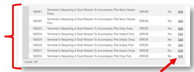
If each of these rules is set as 'error' and 'No', a dual transaction will not be required. To require a dual transaction for the given rule, select edit. Using the drop-down menu. change No to Yes. Then select OK.
